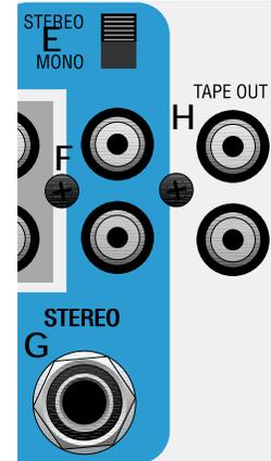
**F. TAPE IN** - Balanced phono (RCA) input jacks designed for use with a tape player, CD player, etc. These jacks are stereo and the full stereo field will be heard when playing prerecorded music. Note: These connectors are set at a constant "line level".
