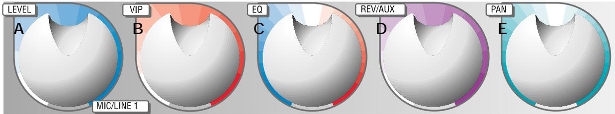
**A. LEVEL** - Adjusts the volume level of the individual channel. Rotating the knob clockwise increases the respective channel's contribution to the "Main Out" mix, while rotating it counterclockwise decreases the volume. Adjust this control after the Passport's master output level volume has been set.
