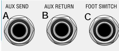
**C. FOOT SWITCH** - The Footswitch connector allows the internal reverb return to be muted, or shut off, through the use of a simple foot operated switch. The footswitch should be wired to connect the tip to sleeve for Off and requires a standard speaker or instrument cable.
