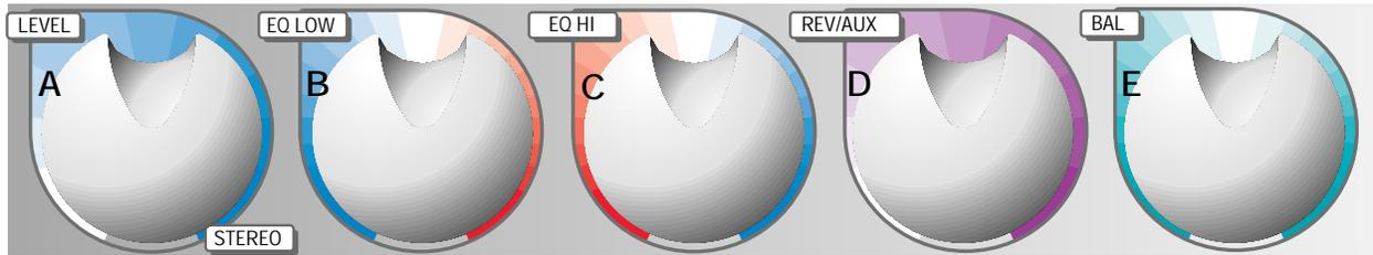
**A. STEREO INPUT LEVEL** - Adjusts the volume level of the stereo input channel. Rotating the knob clockwise increases the stereo input channel's contribution to the "Main Out" mix, while rotating it counterclockwise decreases the volume. Adjust this control after the Passport's master output level volume has been set.
